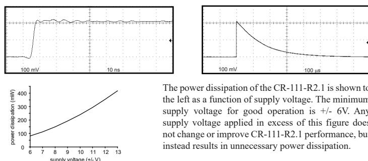
The power dissipation of the CR-111-R2.1 is shown to the left as a function of supply voltage. The minimum supply voltage for good operation is +/- 6V. Any supply voltage applied in excess of this figure does not change or improve CR-111-R2.1 performance, but instead results in unnecessary power dissipation.
