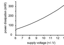
The power dissipation of the CR-113-R2.1 is shown to the left as a function of supply voltage. The minimum supply voltage for good operation is +/- 6V. Any supply voltage applied in excess of this figure does not change or improve CR-113-R2.1 performance, but instead results in unnecessary power dissipation.
