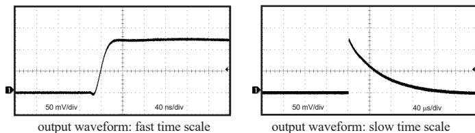
To use an electronic pulser as a test input, apply a square wave (~100 Hz, 50% duty cycle, ~5V p-p) to the 'test in' connection on the instrument. The output should be a series of tail pulses (such as shown in the scope trace above) of alternating positive and negative polarity.
